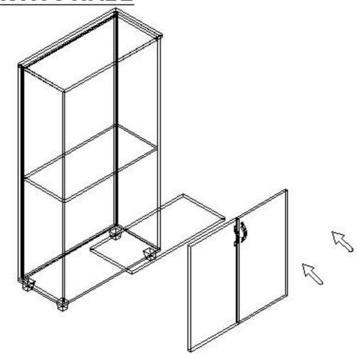
Hinges are fastened to holes of hinge to be on cabinet sides. Hinges are fastened with screws 3,5x18 mm to cabinet doors. Lastly; movable shelfs are placed fastening shelf pims to cabinet sides.
