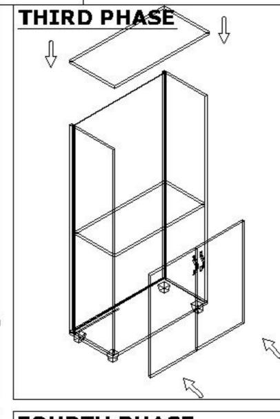
On this phase; Firstly head is placed on clap and concatenated with 4 item screws 3x18 mm from below
