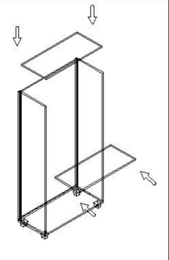
On second phase, backing is passed from ports to be on cabinet sides. Then cabinet head is fastened on clap its below and fixed shelf is fastened to cabinet sides with 4 item minifix.
